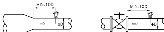
C) Installing on narrower pipe
